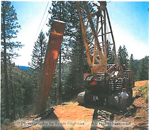
High-lead logging, a common tree-removal process in the Northwest (but not without its problems)
